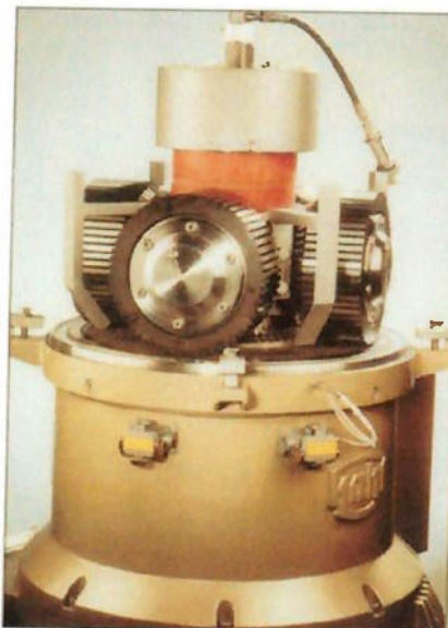
The Pellet Press is used for medium to high pressure extrusion.
