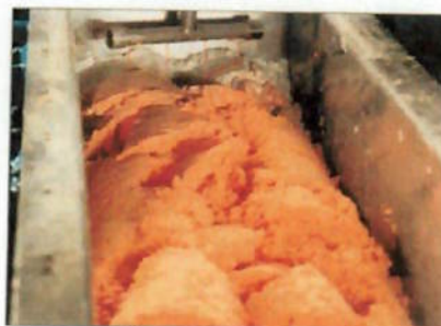
Mixers and kneaders provide the proper powder/liquid mixture for subsequent extrusion.
