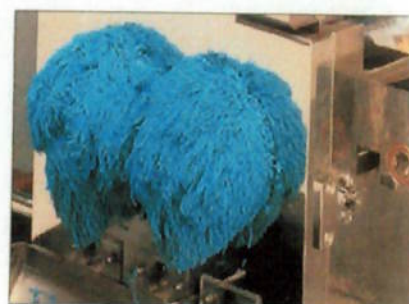
The Twin Dome™ Granulator provides high capacity, low pressure extrusion of powders.
